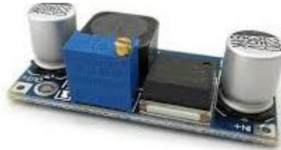
Fig. 6 DC-DC Buck Converter
