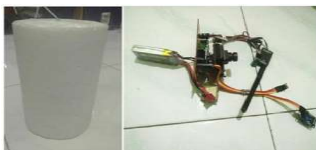
Fig. 5. Transmitter casing and transmitter without casing
